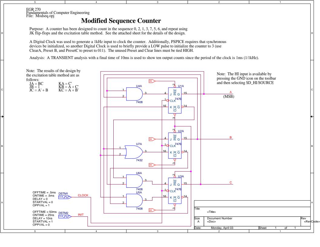
Date/Time run: 04/03 22:32:27 Temperature: 27.0 (A) Modified Sequence Counter with the counting sequence 0,2,1,3,7,5,6 and repeat CLOCK В С COUNT 0s 2ms 4ms 8ms 10ms 6ms
