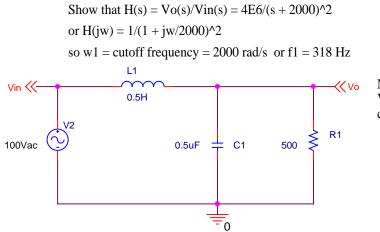
Note that OFFPAGE symbols were added so that Vin and Vo could be conveniently labeled on the circuit.
