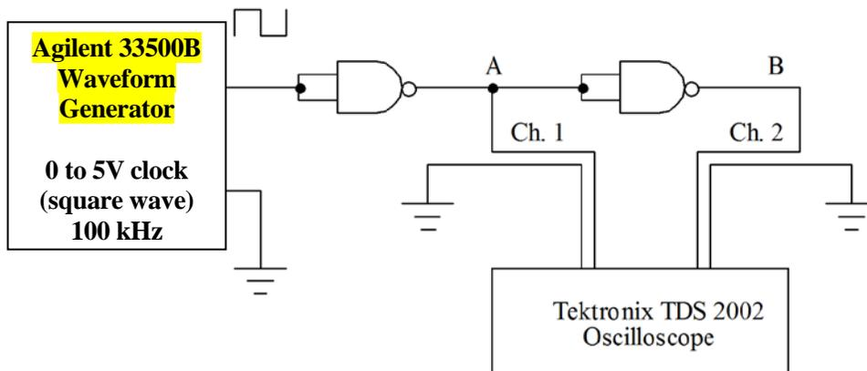
Circuit 2: Measurement of  $t_{PHL}$  and  $t_{PLH}$
