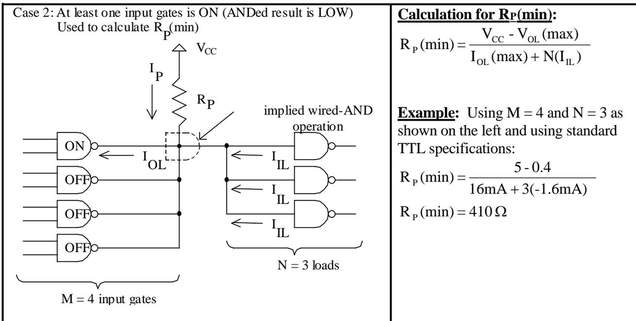
Figure 9 - Calculating the minimum pull-up resistor value
