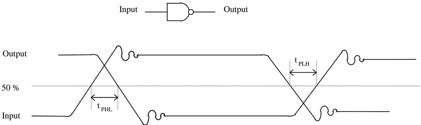
Figure 3: Propagation delay illustration
