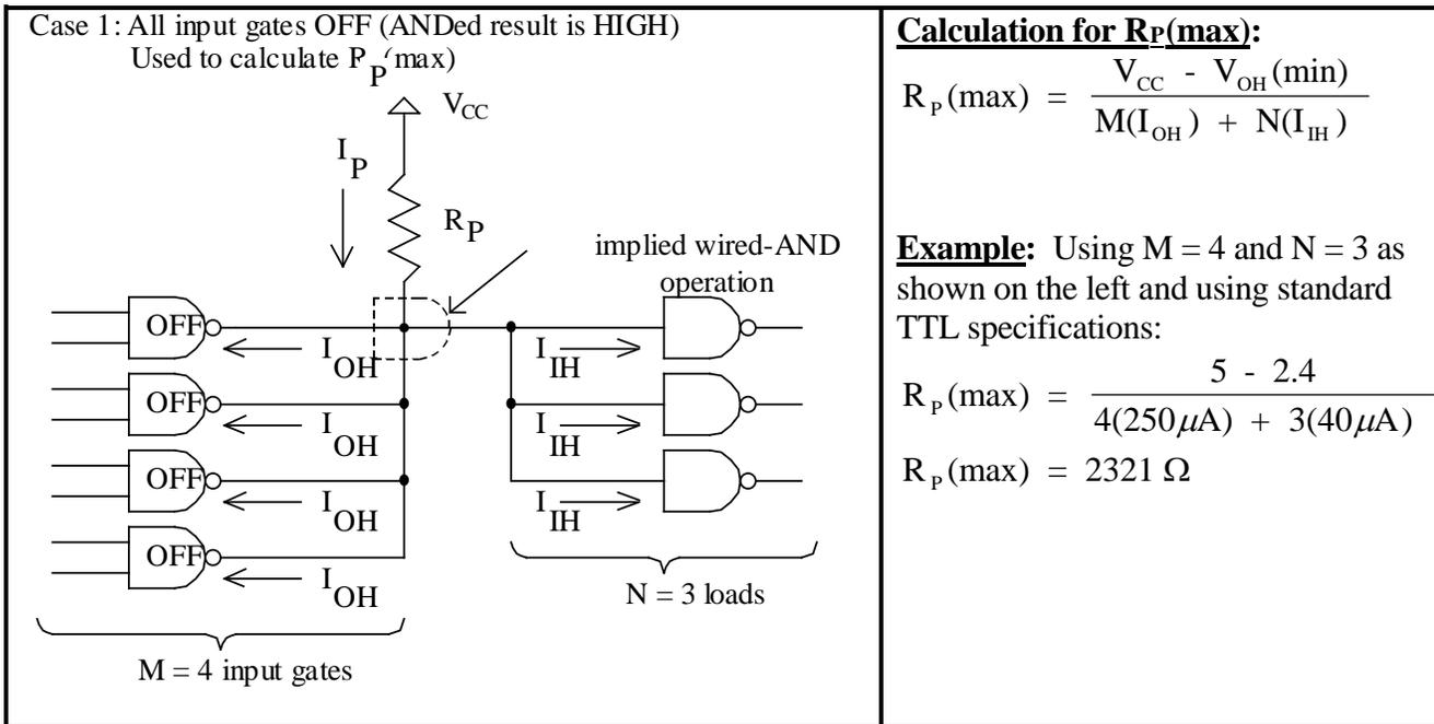
Figure 8 - Calculating the maximum pull-up resistor value
