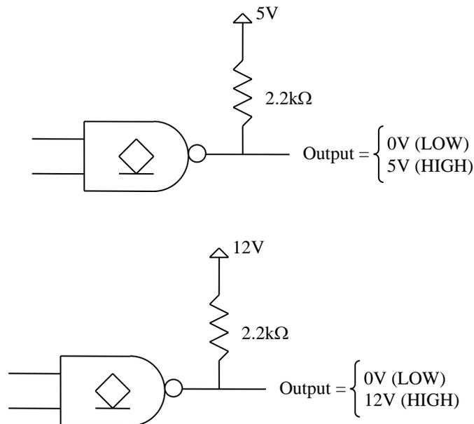
Figure 7: Open-collector gates with 5V and 12V outputs
