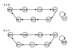
State diagram is the combination of the above two diagrams.
