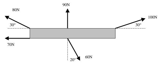
Recalling that angles in polar numbers must be *measured counterclockwise from the positive x-axis*, the sum of the forces above is easily found as follows:
