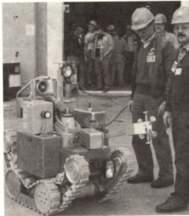
Robots perform tasks in environments that are dangerous for humans. This robot is used for routine inspection, monitoring, and surveillance tasks within areas of a nuclear power plant that are subjected to radiation. (Courtesy of Public Service Electric and Gas Company)
