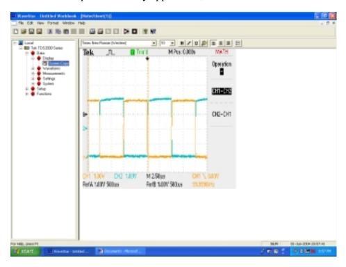
5. A) **Example**: Measuring propagation delay (Channel 1 is the input to an inverter and Channel 2 is the output). Note that the delay can't be seen here, so the transition area is magnified on the next two screen captures.
