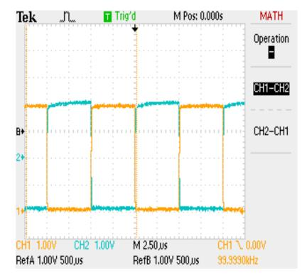
B) Measuring  $t_{PLH}$  (the output is changing from L to H).
