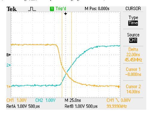
C) Measuring  $t_{PHL}$  (the output is changing from H to L).
