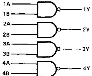
positive logic:  $Y = \overline{A+B}$  or  $Y = \overline{A} + \overline{B}$
